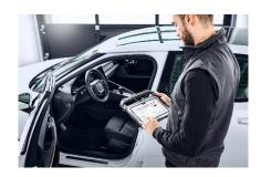
The Smart Scan function of the TechPRO® 2 diagnostic tool provides workshop employees with additional information about the vehicle error codes read.
